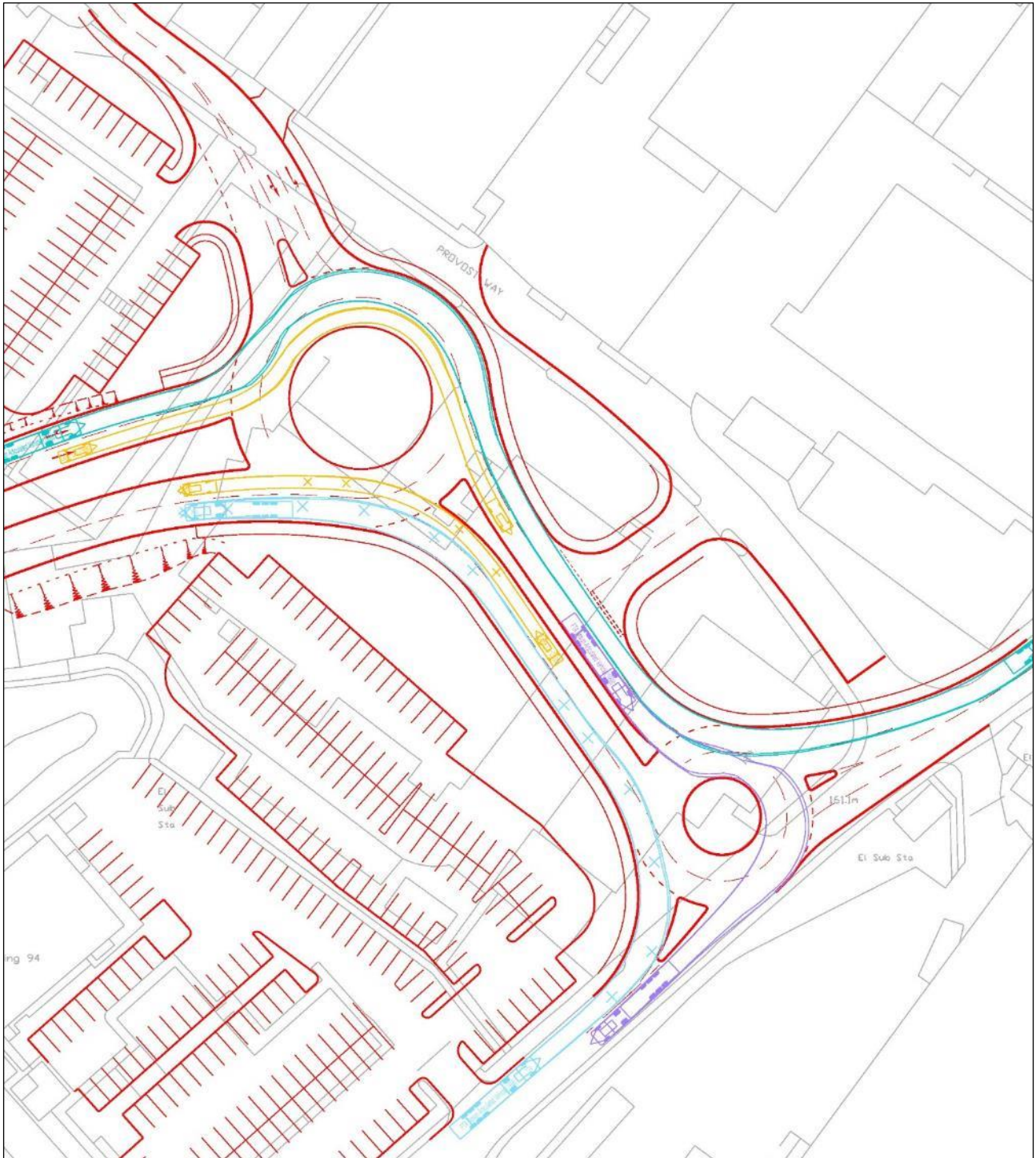
Figure 3.2: Swept Paths - AAR / Provost Way
