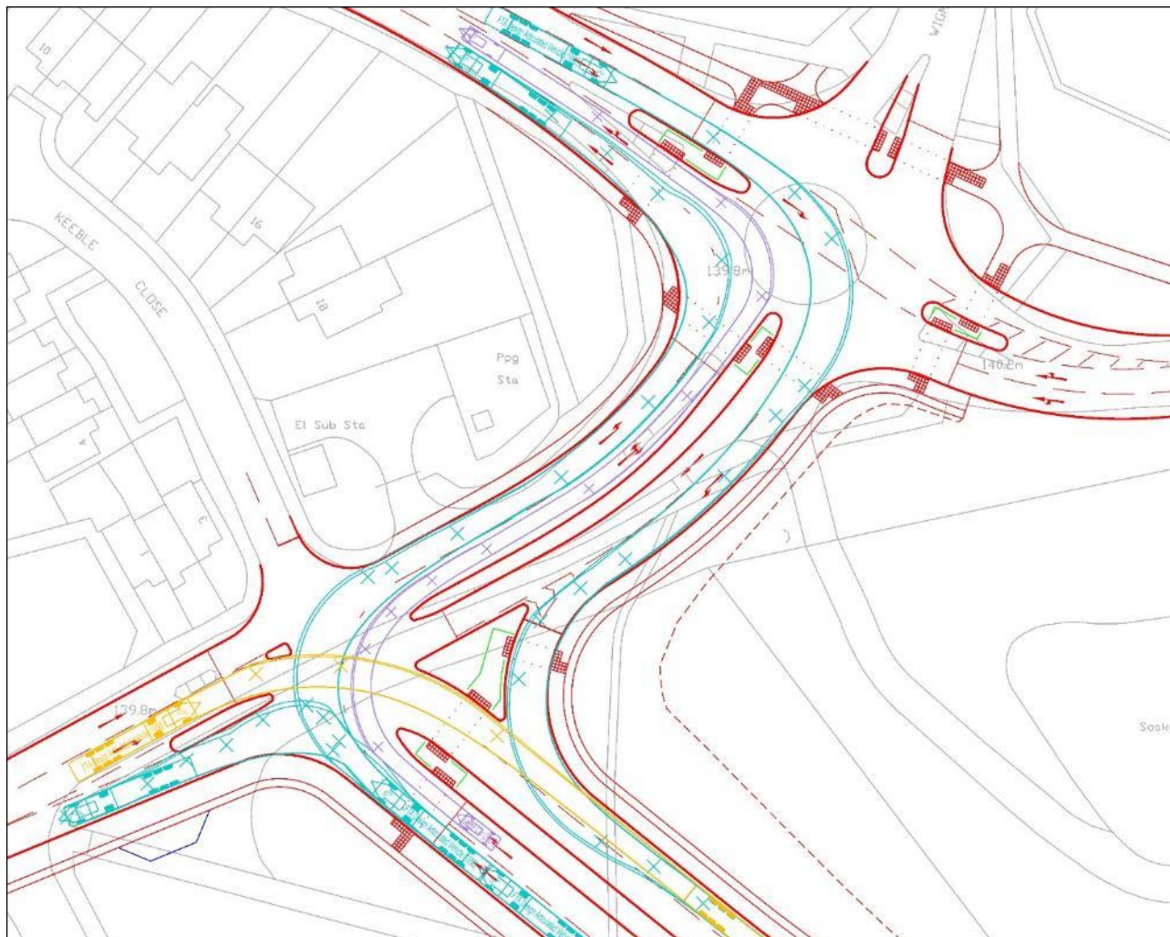
Figure 3.6: Swept Paths - Eaton Green Road Link / Eaton Green Road / Wigmore Lane
